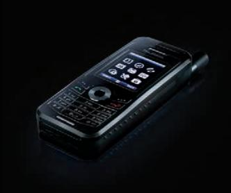
Rugged design Built to exacting standards and using the latest durable polycarbonates for the outside case, it is quite simply, the most durable satellite phone in the market. Thuraya XT's IP54/IK03 rating is a globally recognised standard from the International Electrotechnical Commission, meaning it is splash resistant, dust resistant and shock-proofed.
