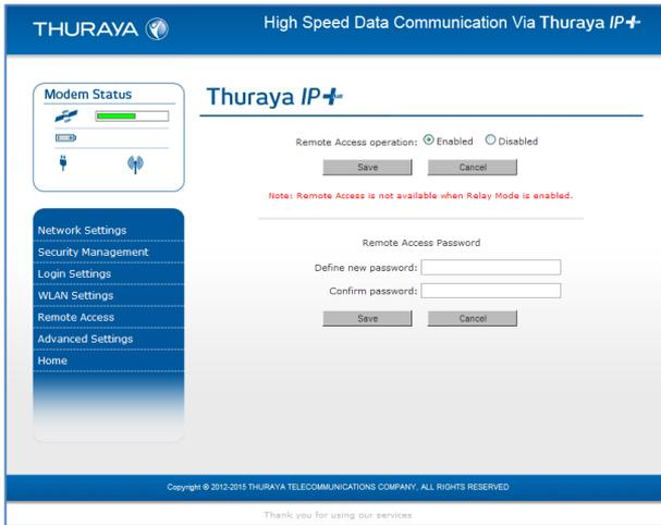
The **Remote Access** screen enables wMMI access from the satellite side of the terminal. To use the feature, select the **Enabled** option, type in a password and select **Save**. Obtain the network IP address from the **Properties** screen and use that in the browser on the remote PC as follows: <http://85.115.79.53:45380> (85.115.79.53 is an example; your terminal address will be different and can change with each PDP session). In general the IP address to use is
