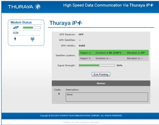
The **Antenna Pointing** screen step can be enabled using the **Antenna Pointing** option on advanced settings screen described above. When this option is **enabled**, the Thuraya IP+ will stop in a pointing mode prior to accessing the network after powering up. This can be useful when optimal pointing is important, such as with fixed installations using an external antenna.
