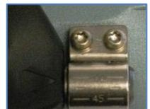
elevation angle correctly set, place the Thuraya IP+ on a flat surface with the antenna facing in the direction of the satellite as determined in step 3.
