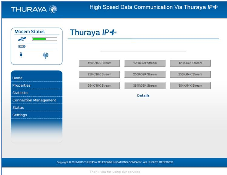
Accessible from the main menu, the **Connection Management** screen allows you to select from nine QoS quick connect buttons. Each button can be customized using the **Details** link on the **Connection Management** screen. The customization parameters for each button are as follows:
